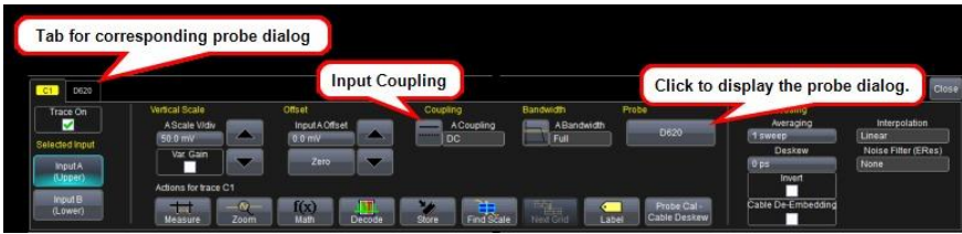
The channel dialog layout showing Input A's ProLink interface controls setup after connection.
