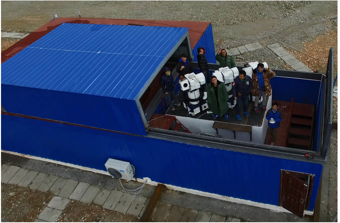
Extended Data Figure 3 | Aerial photograph of the teleportation ground station. Multi-photon sources are prepared in the laboratory on the first floor. Three transmitting antennas are set on a high cement pier and arranged at the same latitude.
