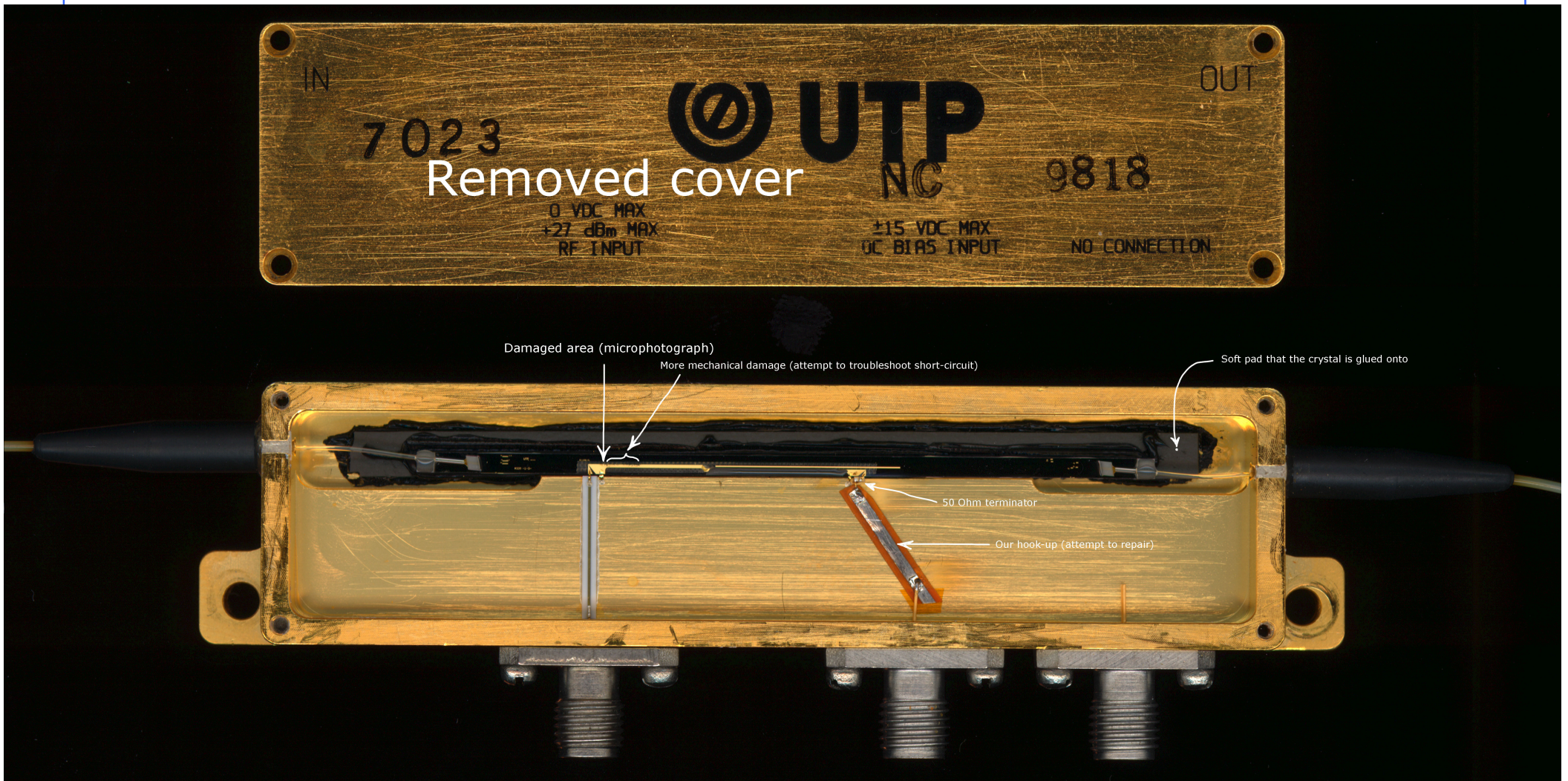
20 GHz travelling-wave phase modulator, 1300 nm (manufacturer: Uniphase)
