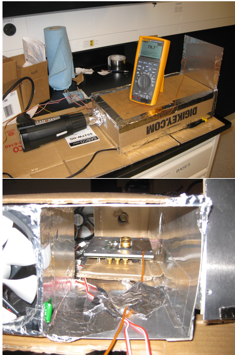
Figure 8.10: Setup for thermal annealing of a group of APDs
