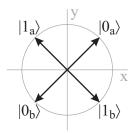
Fig. 1. States configuration for the SARG04 protocol in the case when the states used are physically equivalent to those in the BB84 protocol. The circle represents the equator of the Poincare sphere.
