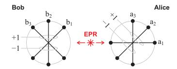
Fig. 5. Possible measurements by Alice and Bob in the Ekert protocol. The circles represent the equator of the Poincare sphere. Measurement bases are denoted by letters with indices; each measurement can yield +1 or -1 result as labeled on the diagram. EPR, source of entangled photon pairs.
