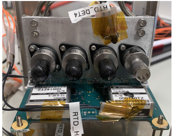
Fig. 1. DM with four capped Si SPADs atop a printed-circuit board providing temperature control and bias voltage.
