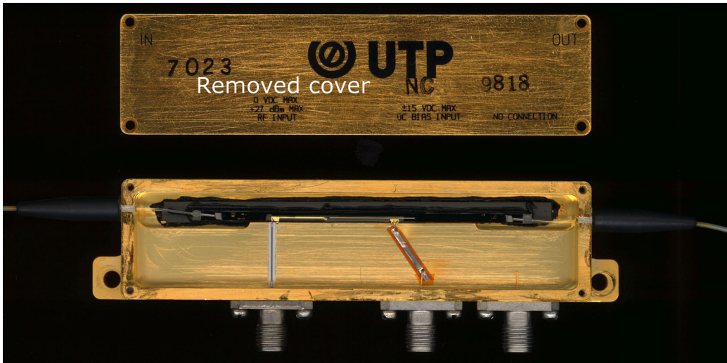
Fig. 35. Lithium niobate phase modulator (JDS Uniphase UTP PM-130-080 travelling-wave 8 GHz, manufactured in 1998), cover removed. Reproduced here in 1:1 scale. Package size 89 \times 23 \times 10 mm (not including protruding elements). The coaxial connectors are of the SMA type.
