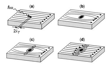
Fig. 29. Schematics of the hotspot-generated and supercurrent-assisted formation of a resistive barrier in an ultrathin and submicrometer-width superconducting stripe, kept at a temperature far below  $T_c$ . The arrows indicate the flow direction of a supercurrent biasing the stripe (reprinted from [151]).
