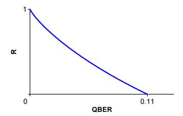
Fig. 36. The available bit rate after privacy amplification as a function of the measured QBER (Eq. 12).
