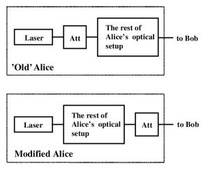
Figure 7. Modification of Alice's set-up.
