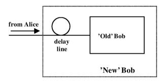
Figure 6. Passive security measures for Bob's set-up.
