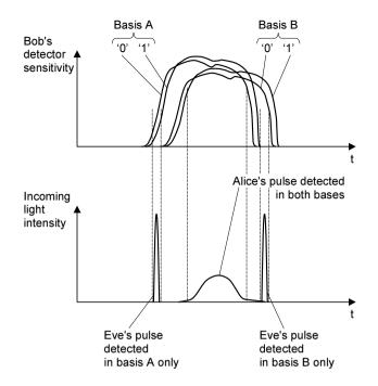
Figure 44. Bob's detection windows shown in the time frame of the incoming light pulses. Bob's detection windows may be shifted relative to each other between the bases and bit values. This does not affect normal operation: Alice's pulse is shown arriving during the time when all the windows overlap. However, if well defined non-overlapping zones exist like on this drawing, Eve may exploit them to choose the basis (her pulses shown on the diagram), and also the bit value.
