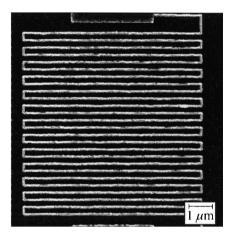
Fig. 28. A scanning electron microscope image of a  $10 \times 8 \ \mu m^2$ , 10 nm thick meandertype SSPD, NbN superconducting stripe on a sapphire substrate. The stripe width is ~130 nm and the filling factor f = 0.2 (reprinted from [151]). This filling factor is due to a particular technology used for fabricating the depicted sample, and is not the highest achievable: f ~0.5 is possible with other technologies.
