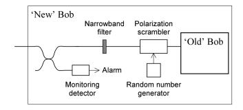
Figure 45. Additional security equipment needed to protect Bob (who is using passive basis choice) from the faked states attack described in this paper. In addition to what is shown on the diagram, Bob must match the timing of his detection windows to each other exactly.
