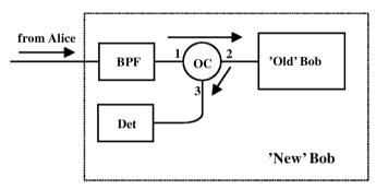
Figure 10. Active/passive security measures for Bob's set-up with the B92 protocol, with low additional losses and weaker requirements to the sensitivity of the alarm detector.
