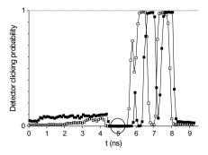
FIG. 7. Detector model 2. Sensitivity curves for the 0 (open squares) and 1 (filled squares) time slots, at mean number of photons at the APD  $\mu$ =500. In the encircled time range (4.65–5.30 ns) the clicking probability in both detectors measured exactly zero (0 counts registered per >10<sup>5</sup> gates). Unfortunately the time reference in this plot is not accurately matched with that in Fig. 6, and the curves' features cannot be directly compared between the two figures.
