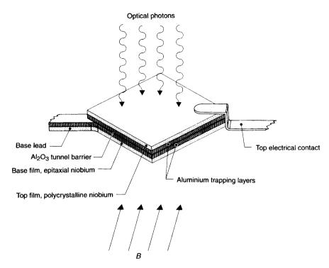
Fig. 25. A diagram of a  $20 \times 20 \ \mu m$  STJ device (not to scale). It was fabricated from a 'sandwich' of Nb/Al/Al<sub>2</sub>O<sub>3</sub>/Al/Nb deposited on polished sapphire. The base and top niobium films have a thickness of 100 nm; both the aluminium films are 120 nm thick; the aluminium oxide barrier has a thickness of ~1 nm (reprinted from [138]).
