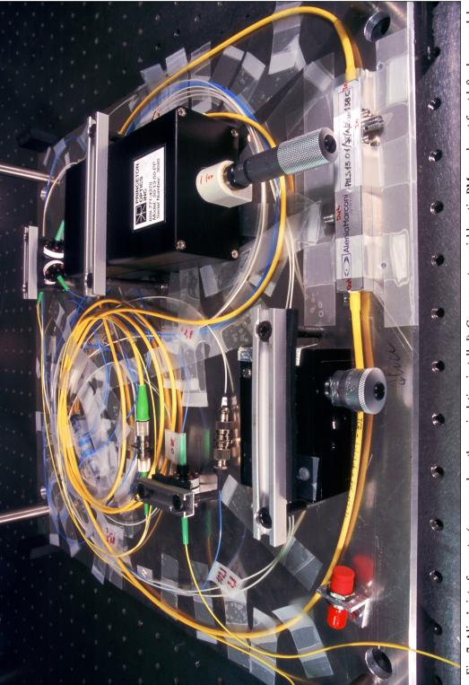
Fig. 7. Alice's interferometer (uncovered, no thermoisolation installed). Components: variable ratio PM coupler, at front left; phase modula-tor; at front right; polarizer, at middle left; variable delay line, at middle right; polarization combiner, at back right. Laser module not shown.
