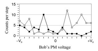
Fig. 17. Interference curves for "0" and "1" time slots, plotted from data measured in a single run of stage 1 phase adjustment. The  $2\pi$  phase range was scanned in 16 steps, and on average 150 counts were collected on stage 1. Curve with solid points is for "0" time slot and curve with hollow points is for "1" time slot.
