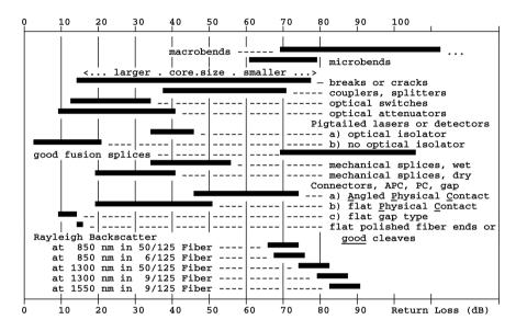
Appendix B: Reflection coefficients for different fibre-optic components
