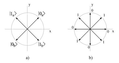
Fig. 39. States configuration for QKD protocols robust to PNS attack: (*a*) SARG04 protocol: two pairs of non-orthogonal states on the equator of the Poincare sphere, physically equivalent to the states used in the BB84 protocol; (*b*) bit encoding in a PNS-resistant protocol using four bases (reprinted from [65]).
