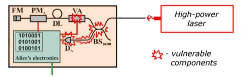
Fig. 41. Optical parts potentially vulnerable to a high-power damage attack in Stucky's *et al.* setup [63]. Alice's part of the optical scheme is shown in the diagram (FM, Faraday mirror;  $PM_A$ , phase modulator; DL, delay line; VA, variable attenuator;  $D_A$ , detector;  $BS_{10/90}$ , asymmetric beamsplitter).
