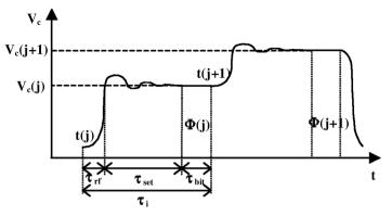
Figure 2. Transmission cycle and time parameters.
