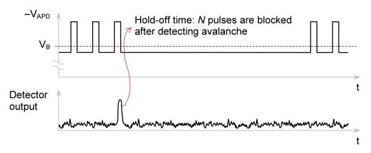
Fig. 31. Principle of afterpulse blocking.
