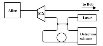
Figure 1. General structure of eavesdropping set-up.
