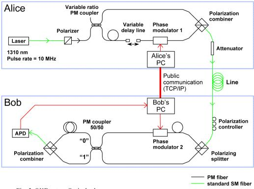
Fig. 5. QKD setup. Optical scheme.
