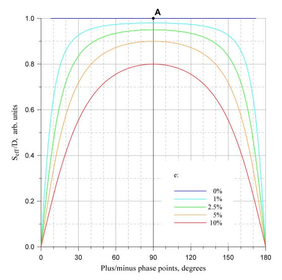
Fig. 20. Effective slope to statistical deviation ratio  $S_{eff}/D$  as a function of  $\varphi$  (Eq. 10) plotted for several values of base level *e* typical for quantum cryptography setups (*e*=0.01 (1%) to *e*=0.1 (10%)) as well as for *e*=0. Note that the Gaussian approximation assumed in the derivation may not hold near 0° and 180° for the *e*=0 curve. **A**: point used for all derivations in the above paper.
