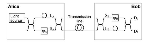
Fig. 2. Interferometric QKD channel with phase coding. The two arms of the Mach-Zehnder interferometer are multiplexed into a single transmission line.
