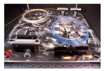
Fig. 16. Bob's interferometer. All components are mounted on a 400x400x6 mm aluminium plate, and their fiber pigtails are affixed to the plate surface with pieces of adhesive tape. Everything is covered by custom-cut pieces of foam insulation (not shown on the photo) and mounted inside a box. Alice's interferometer is similar.
