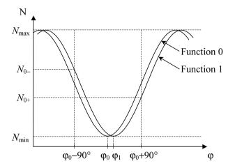
Fig. 14. Illustration of phase adjustment at stage 2. Only the interference curve for "0" time slot is shown.
