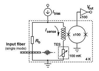
Fig. 27. Schematic of a TES device biasing and readout. The voltage bias for the device is provided by a room-temperature current source ( $I_{\text{bias}}$ ) and a 100 µOhm shunt resistor ( $R_{\text{b}}$ ) at 4 K. The device signal  $I_{\text{sense}}$  is amplified by a 100-element array of dc-SQUID amplifiers and processed with room-temperature pulseshaping electronics (reprinted from [145]).
