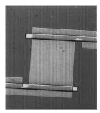
Fig. 26. Photograph of a TES with  $18 \times 18 \,\mu\text{m}$  W sensor and Al voltage rails. The thickness of the W film deposited on a Si substrate is 40 nm (reprinted from [144]).
