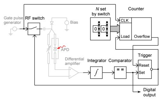
Fig. 32. Hardware implementation of afterpulse blocking. Grayed out parts are those inherited from the SPD without afterpulse blocking (Fig. 30); parts drawn in black lines form the afterpulse blocking circuitry.
