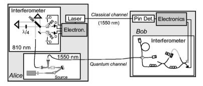
Figure 42. Reprinted from [50]: asymmetric system for quantum key distribution utilizing photon pairs (PBS, polarizing beam splitter; D, single-photon detector;  $\lambda/4$ , quarter-wave plate; HSM, half-silvered mirror).
