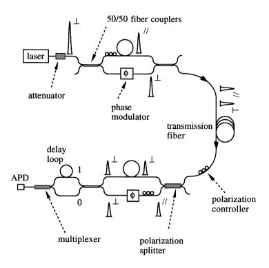
Fig. 3. Reprinted from [24]: interferometric quantum cryptography scheme.
