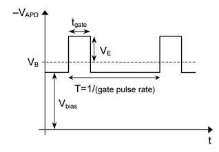
Fig. 23. Voltage at the APD in the gated mode of operation. The expected time of photon arrival is periodic in the depicted case.
