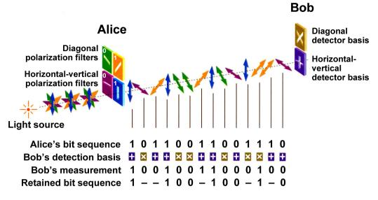
Fig. 1. Principle of the BB84 protocol (reprinted from [20]).
