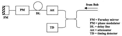
Figure 5. Alice's set-up in the 'plug & play' scheme.
