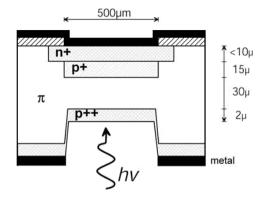
Fig. 21. Schematic cross-section of Si APD with reach-through structure developed by McIntyre and Webb in 1970s (reprinted from [108]).
