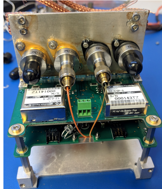
Figure 3: SPAD flight module stacked on control module of the CAPSat annealing payload.
